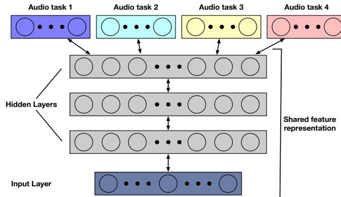
Fig. 1. Architecture of the multi-task deep neural network.
