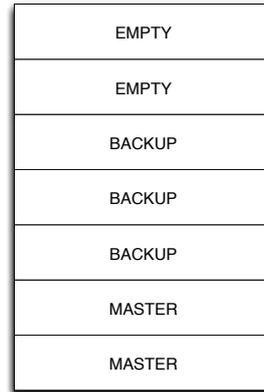
**Figure 2: Buffer Management:** the figure shows a buffer with a size equal to 7, with 2 master copies in it. In this case, the node will advertise 5 available slots.
