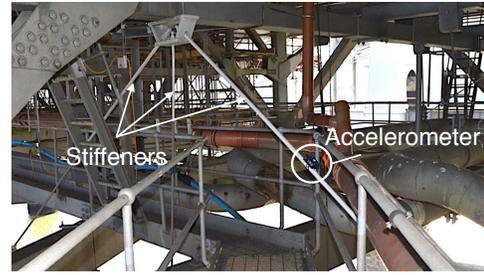
**Figure 3. Accelerometer attached to a stiffening member.**
