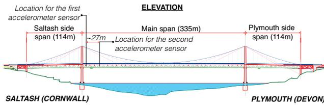
**Figure 4. South elevation diagram showing accelerometer locations.**
