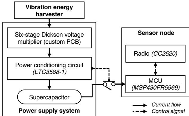
**Figure 1. Hardware architecture of the energy-harvesting sensor node.**
