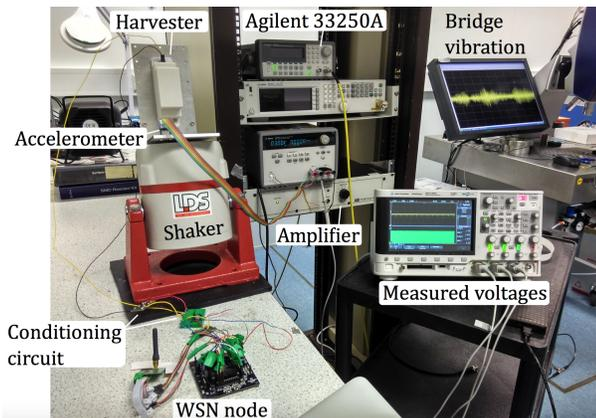
Figure 16. Experimental setup.
