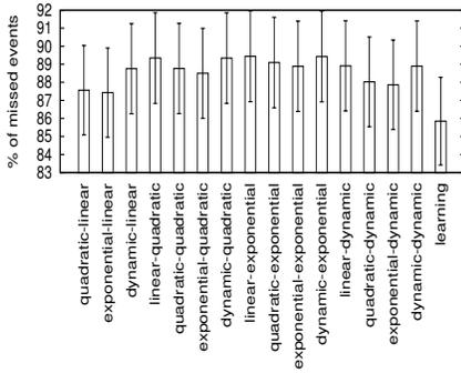
Figure 10: Accuracy of the adaptation schemes for accelerometer.
