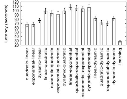
Figure 12: Latency of the adaptation techniques for accelerometer.
