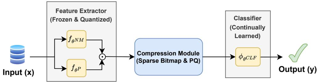
**Figure 2: The system overview.** LifeLearner consists of the frozen/quantized feature extractor, the continually learned classifier, and the compression module based on sparse bitmap and PQ. The compression module takes the feature extractor’s outputs (activations) as inputs and compresses them to be saved as latent replay samples.
