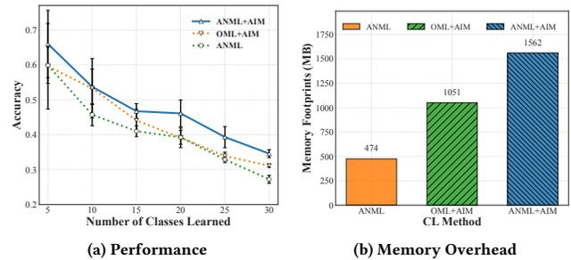
**Figure 1: Preliminary analysis of the prior Meta CL methods (i.e., ANML, OML+AIM, ANML+AIM). (a) shows the CL accuracy degradation of the Meta CL methods after learning  $c$  number of classes on CIFAR-100 [47]. (b) shows the memory footprint needed to run the Meta CL methods on MiniIma-geNet [95] with a batch size of 8.**
