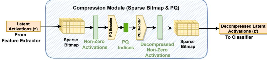
**Figure 3: The overview of our compression module. It consists of (1) a sparse bitmap to filter out zero from activations or to reconstruct decompressed activations from non-zero activations, (2) a PQ encoder that further compresses non-zero activations into PQ indices, and (3) a PQ decoder that decompresses PQ indices back into decompressed non-zero activations.**
