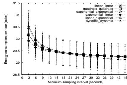
Figure 8. Energy consumption vs minimum sampling interval for accelerometer sensor.
