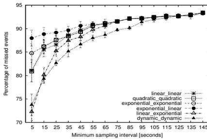
Figure 9. Percentage of missed events vs minimum sampling interval for microphone sensor.
