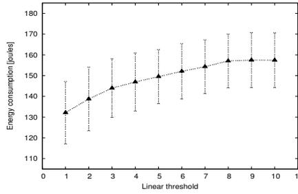
Figure 2. Energy consumption vs linear threshold for Bluetooth sensor.
