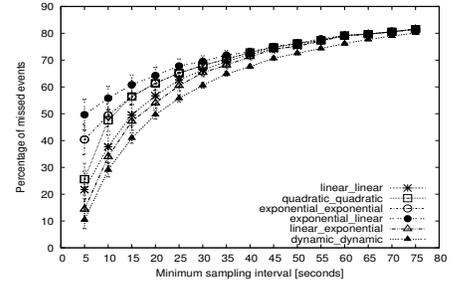
Figure 3. Percentage of missed events vs minimum sampling interval for Bluetooth sensor.
