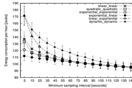
Figure 10. Energy consumption vs minimum sampling interval for microphone sensor.
