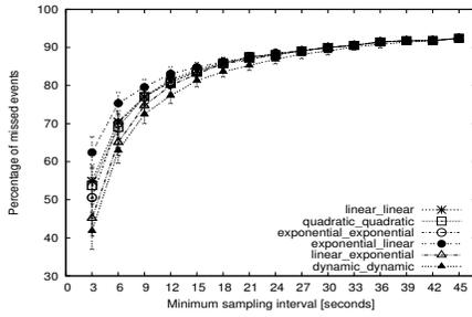
Figure 7. Percentage of missed events vs minimum sampling interval for accelerometer sensor.
