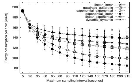
Figure 6. Energy consumption vs maximum sampling interval for Bluetooth sensor.
