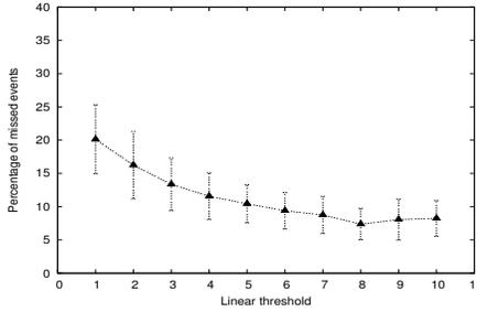
Figure 1. Percentage of missed events vs linear threshold for Bluetooth sensor.
