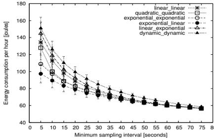
Figure 4. Energy consumption vs minimum sampling interval for Bluetooth sensor.
